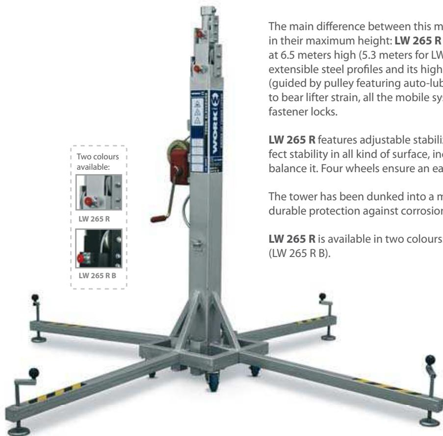
The main difference between this model and the LW 255 R lies in their maximum height: **LW 265 R** can lift loads of 220 kg at 6.5 meters high (5.3 meters for LW 255 R) thanks to its five extensible steel profiles and its high traction resistant cable (guided by pulley featuring auto-lubricated bearing). In order to bear lifter strain, all the mobile system is fixed with safety fastener locks.
